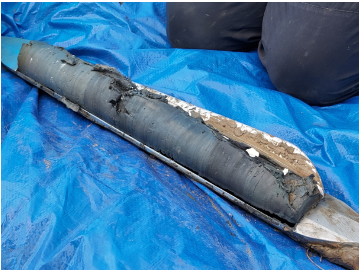
The Russian corer head full of lagoon sediments (and of palaeoenvironmental
